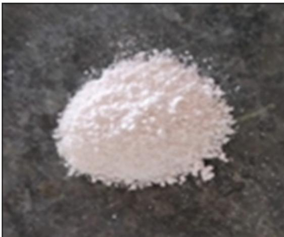
Figure 1: Optical image of combustion-derived  $\text{CaTiO}_3$ .
