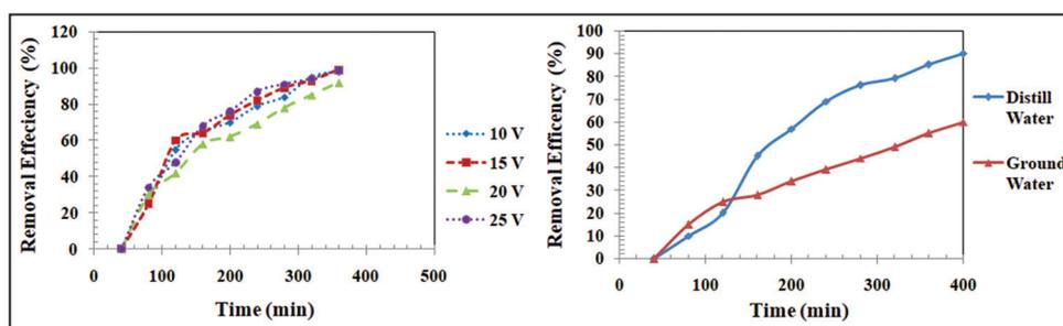
**Figure 5:** Impact of applied voltage on the removal of fluoride in an EC batch reactor, examining the variation in conductivity over time of 10 mg/L.
