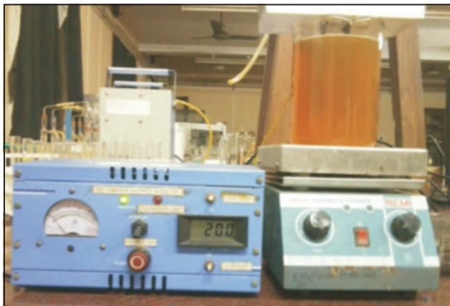
**Figure 1:** An EC batch reactor and experimental equipment were used to eliminate fluoride.
