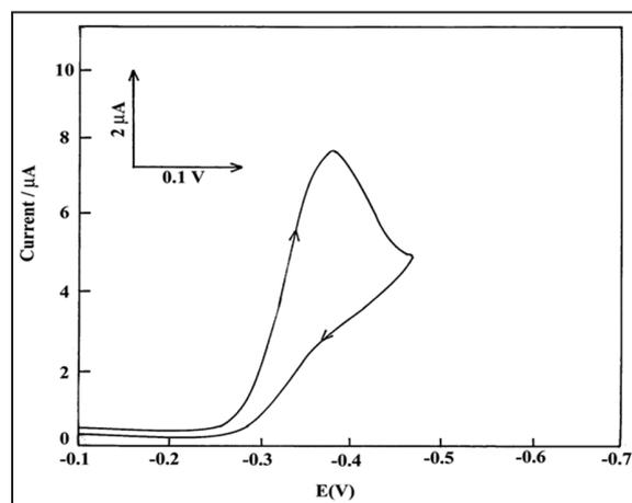
**Figure 1:** Cyclic voltammogram of pindone at pH 4.0 concentration: 0.25 mM, scan rate:  $40 \text{ mVs}^{-1}$ .
