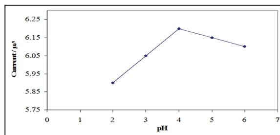
Figure 4: Effect of pH on pindone solution at hanging mercury drop electrode.
