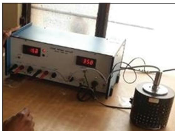
**Figure 1:** Experimental set-up of DC conductivity measurement.
