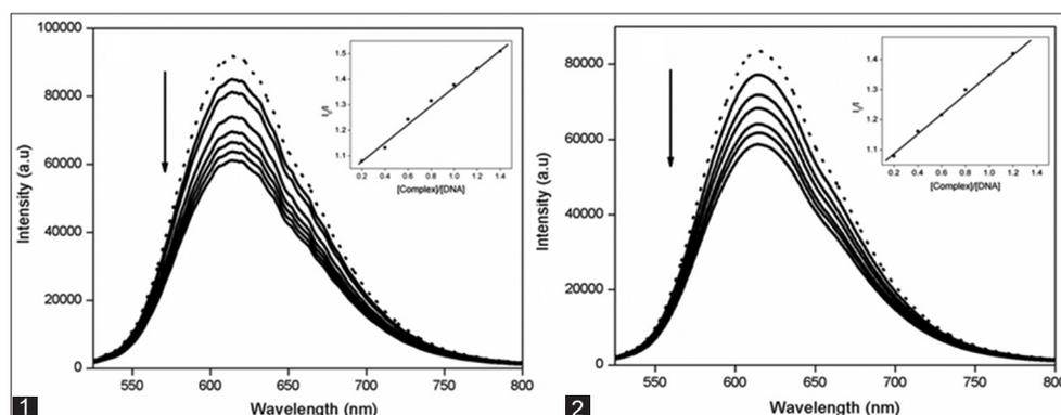
**Figure 2:** Emission spectra of ethidium bromide bound to DNA in the absence (dotted line) and the presence (dashed line) of complexes 1 and 2. Arrow (↓) shows the intensity changes upon increasing the concentration of the complex. Inset: Stern–Volmer quenching curves.
