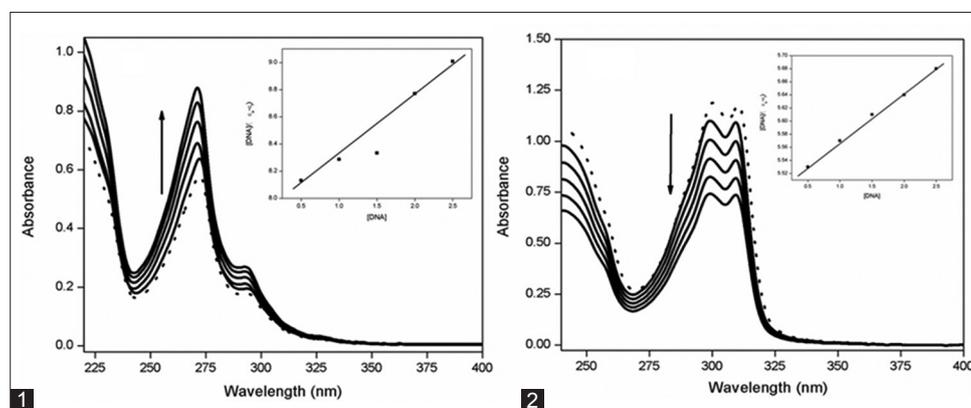
**Figure 1:** Absorption spectral traces on addition of calf thymus (CT)-DNA to complexes 1 and 2 (shown by arrow). Inset plot of  $[DNA]/(\epsilon_a - \epsilon_f)$  versus  $[DNA]$  for absorption titration of CT-DNA with complexes.
