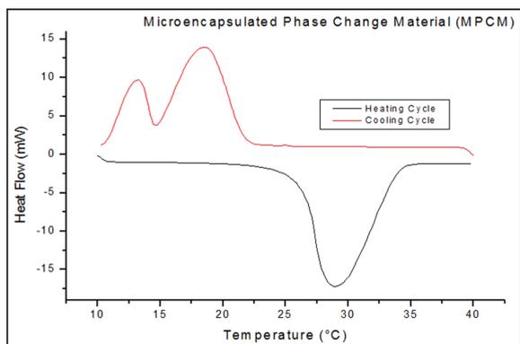
**Figure 2:** Differential scanning calorimetry thermogram of microencapsulated phase change materials.
