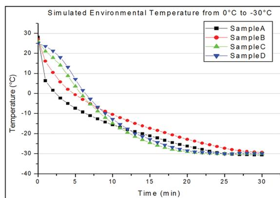
**Figure 6:** Temperature of the comfort pads when subjected to simulated environmental temperature from 0°C to -30°C
