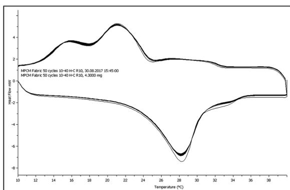
**Figure 4:** Differential scanning calorimetry plot of microencapsulated phase change materials fabric subjected to 50 heating and cooling cycles.
