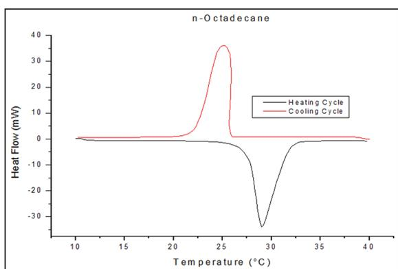
**Figure 1:** Differential scanning calorimetry thermogram of n-Octadecane (phase change materials).
