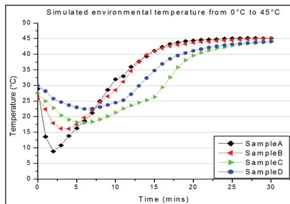
**Figure 5:** Temperature of the comfort pads when subjected to simulated environmental temperature from 0°C to +45°C at 65% relative humidity.
