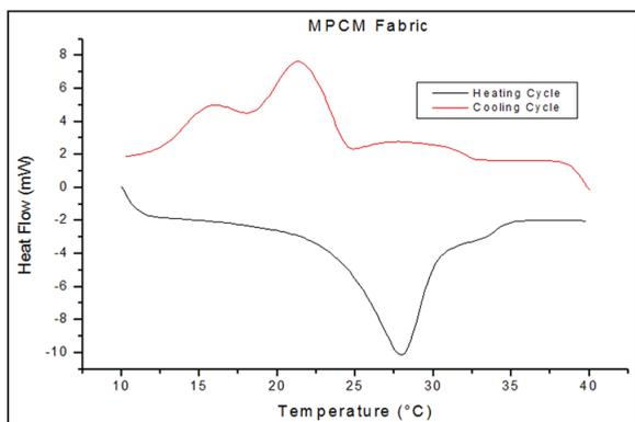
**Figure 3:** Differential scanning calorimetry thermogram of microencapsulated phase change materials coated fabric.
