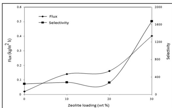
**Figure 8:** Zeolite concentration versus flux and selectivity of sodium alginate-gelatin blend membranes at azeotropic composition.
