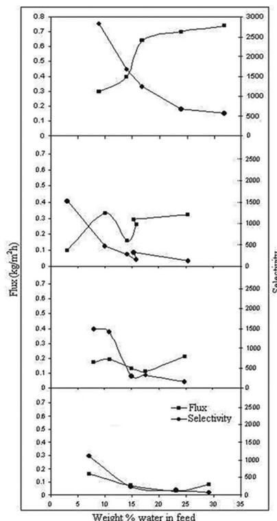
**Figure 7:** Effect of feed compositions on pervaporation performance of (a) sodium alginate-gelatin (SA-GL)-0; (b) SA-GL-10; (c) SA-GL-20; (d) SA-GL-30 incorporated zeolite cross-linked membranes.
