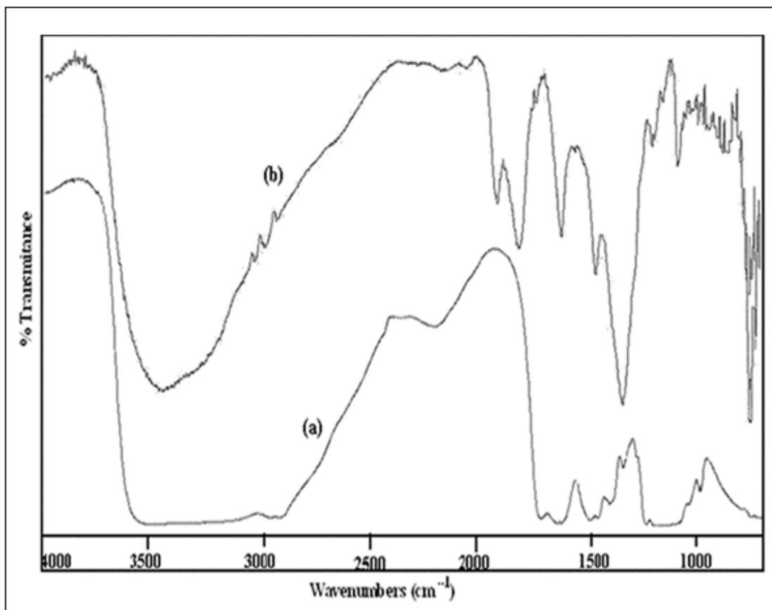
Figure 2: Fourier transform-infrared patterns of (a) sodium alginate-gelatin (SA-GL)-0; (b) SA-GL-30 cross-linked membranes.
