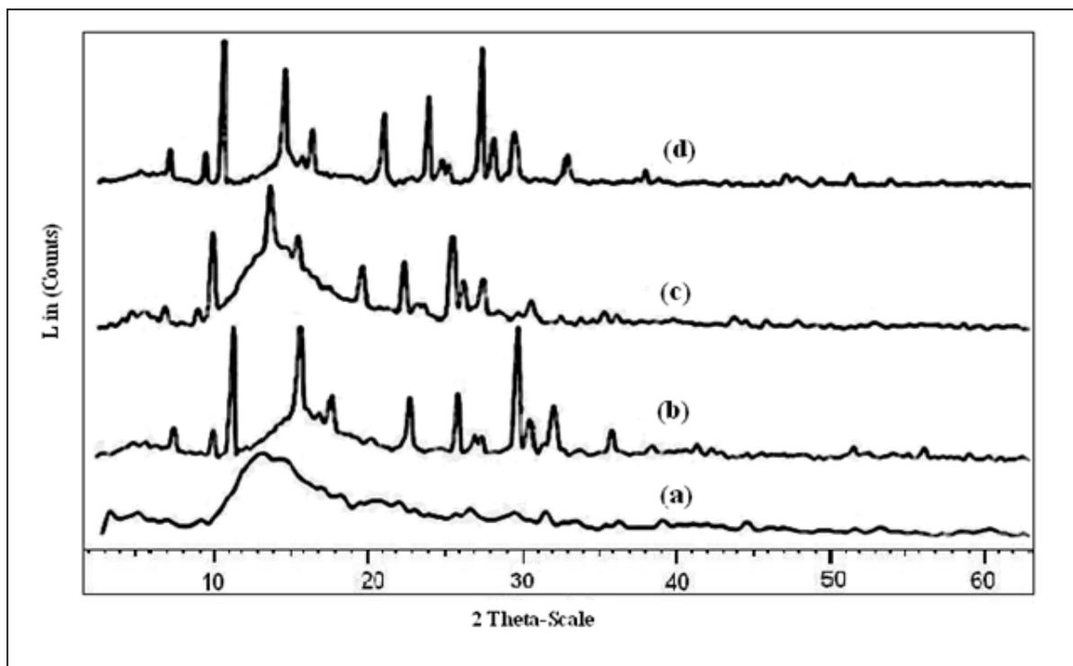
**Figure 3:** Wide angle X-ray diffraction patterns of zeolite filled sodium alginate-gelatin (SA-GL) blend membranes: (a) SA-GL-0; (b) SA-GL-10; (c) SA-GL-20; (d) SA-GL-30.
