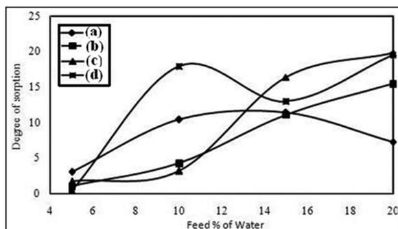
**Figure 6:** Plots of degree of sorption versus percentage of water in the feed (a) sodium alginate-gelatin (SA-GL)-0; (b) SA-GL-10; (c) SA-GL-20; (d) SA-GL-30 incorporated zeolite cross-linked membranes.
