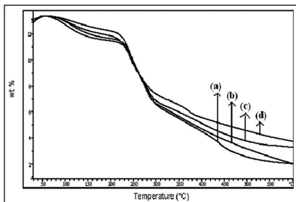
**Figure 5:** Thermogravimetric analysis of (a) sodium alginate-gelatin (SA-GL)-0; (b) SA-GL-10; (c) SA-GL-20; (d) SA-GL-30.
