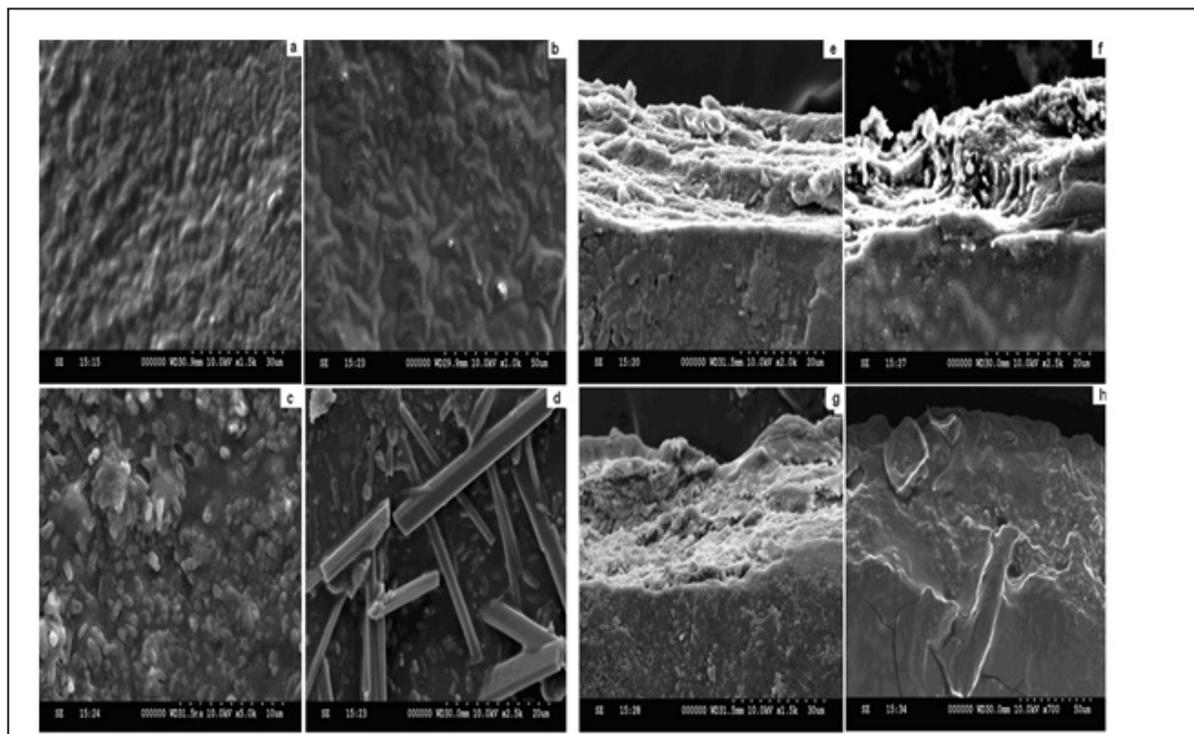
**Figure 4:** (A). Scanning electron microscopy (SEM) pictures surfaces of the: (a) Sodium alginate-gelatin (SA-GL)-0; (b) SA-GL-10; (c) SA-GL-20; (d) SA-GL-30. (B) SEM pictures of the (cross section): (e) SA-GL-0; (f) SA-GL-10; (g) SA-GL-20; (h) SA-GL-30.
