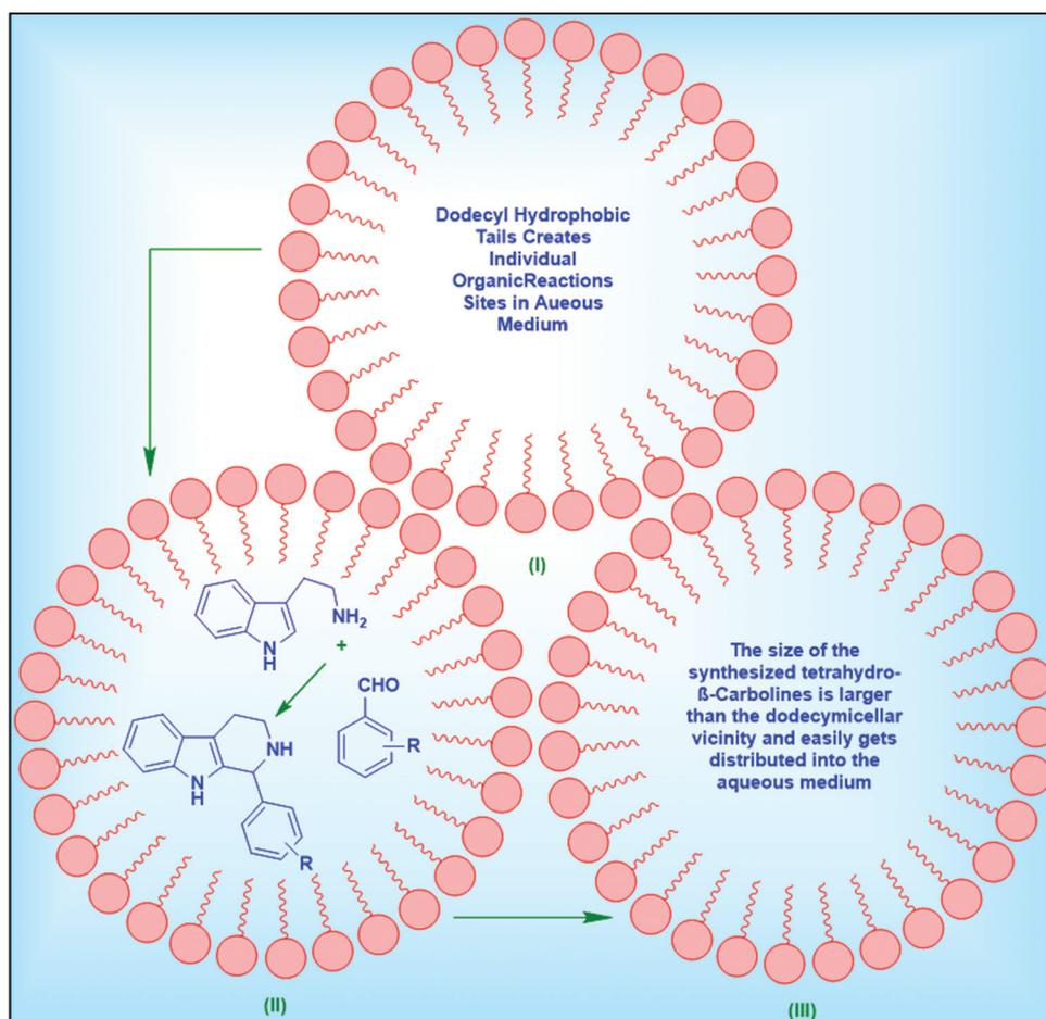
**Figure 2:** Surfactant and Lewis acidic strategy of ferric dodecyl sulfonate catalyst in the synthesis of tetrahydro- $\beta$ -carbolines.
