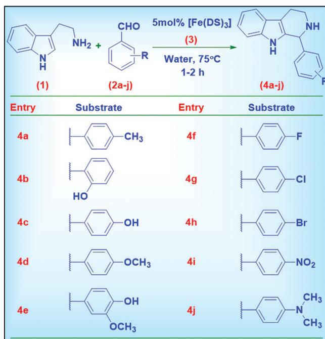
Scheme 1: Synthesis of ferric dodecyl sulfonate catalyzed tetrahydro- $\beta$ -carboline derivatives.
