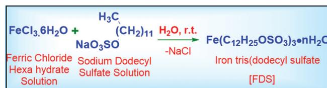
**Scheme 2:** *In situ* preparation of ferric dodecyl sulfonate catalyst.
