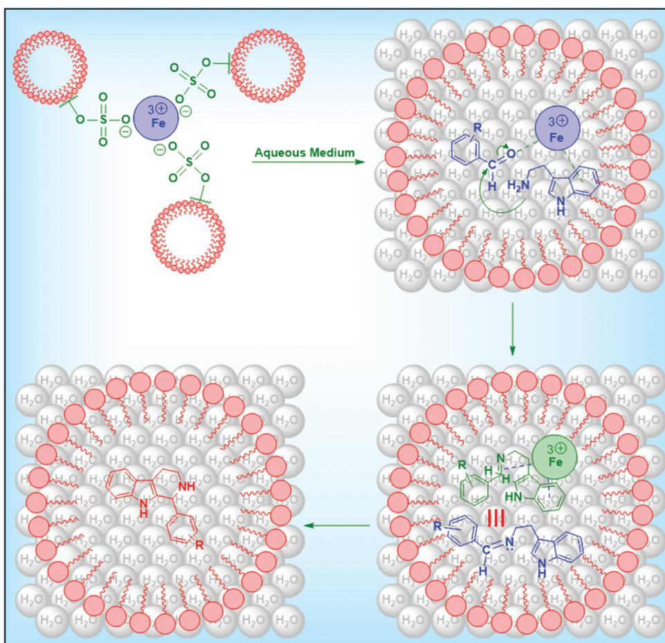
**Figure 1:** Mechanistic approach for ferric dodecyl sulfonate-mediated synthesis of tetrahydro- $\beta$ -carboline derivatives.
