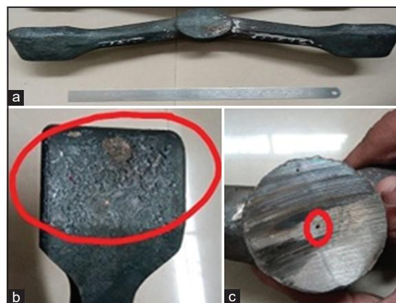
**Figure 9:** (a) The Investment casted specimen, (b) Deposition of PLA vapor on to the shell and (c) Occurred piping defect exactly at the center of the boss
