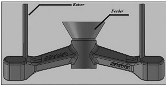
Figure 2: Specimen with the feeder placed exactly over the pattern
