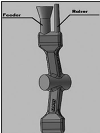
Figure 3: Specimen with feeder and raiser are placed at the top most point
