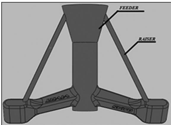
Figure 4: Specimen with feed system placed exactly at the center of the specimen and the raiser were placed at an angle
