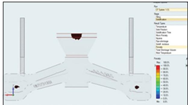
Figure 5: Analysis result for porosity in Case I.
