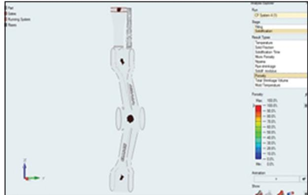
Figure 6: Analysis result for porosity in Case II.
