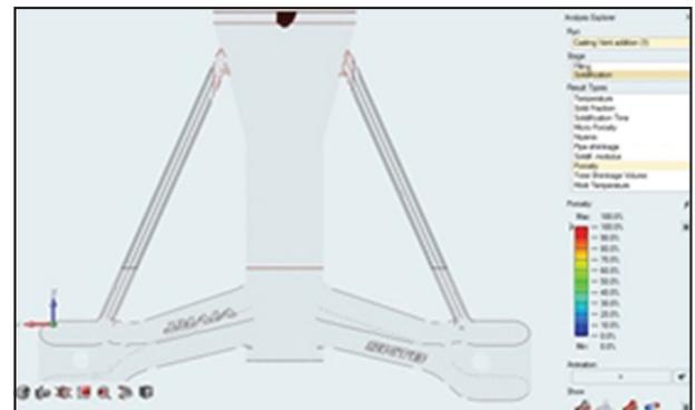
Figure 7: Analysis result for porosity in Case III.
