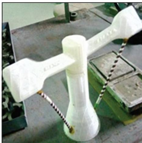
**Figure 8:** The 3D printed casting system
