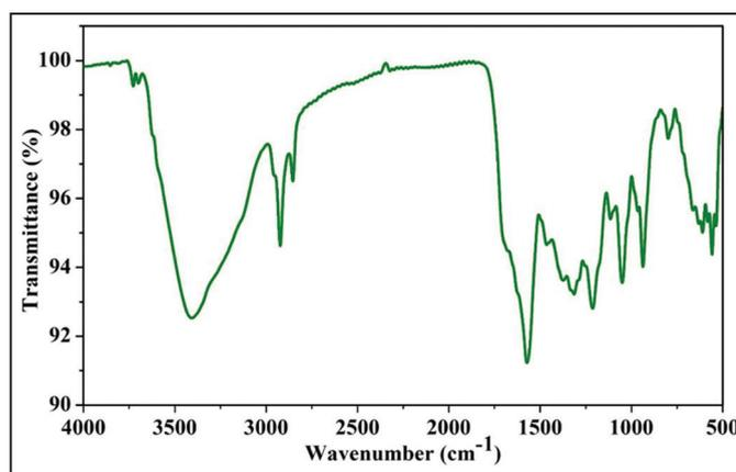
**Figure 1:** The FTIR spectrum of PPY/SnO<sub>2</sub>/SWCNTs. FTIR: Fourier transform infrared spectroscopy, PPY: Polypyrrole, SnO<sub>2</sub>: Tin oxide, SWCNTs: Single-walled carbon nanotubes.
