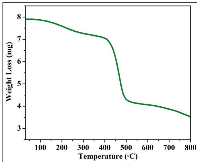
Figure 4: The TGA curve of PPy/SnO<sub>2</sub>/SWCNTs. TGA: Thermogravimetric analysis, PPy: Polypyrrole, SnO<sub>2</sub>: Tin oxide, SWCNTs: Single-walled carbon nanotubes.
