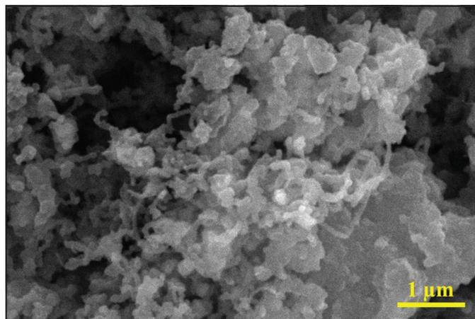
**Figure 3:** The SEM image of PPY/SnO<sub>2</sub>/SWCNTs. SEM: Scanning electron microscopy, PPY: Polypyrrole, SnO<sub>2</sub>: Tin oxide, SWCNTs: Single-walled carbon nanotubes.
