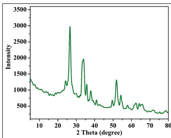
**Figure 2:** The XRD spectrum of PPY/SnO<sub>2</sub>/SWCNTs. XRD: X-ray diffraction, PPY: Polypyrrole, SnO<sub>2</sub>: Tin oxide, SWCNTs: Single-walled carbon nanotubes.
