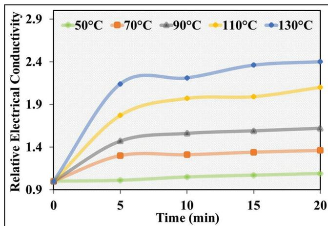
Figure 5: Relative electrical conductivity of PPy/SnO<sub>2</sub>/SWCNTs under isothermal aging condition. PPy: Polypyrrole, SnO<sub>2</sub>: Tin oxide, SWCNTs: Single-walled carbon nanotubes.
