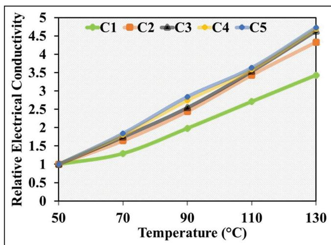
**Figure 6:** Relative electrical conductivity of PPy/SnO<sub>2</sub>/SWCNTs under cyclic ageing condition. PPy: Polypyrrole, SnO<sub>2</sub>: Tin oxide, SWCNTs: Single-walled carbon nanotubes.
