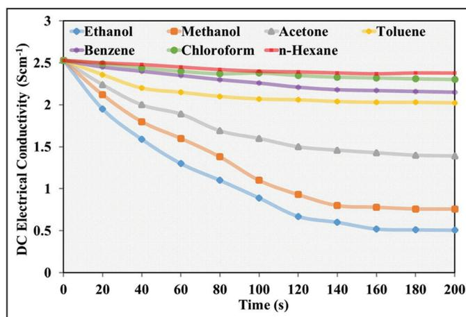
**Figure 7:** The change in conductivity of PPy/SnO<sub>2</sub>/SWCNTs sensor in different organic vapours with respect to time. PPy: Polypyrrole, SnO<sub>2</sub>: Tin oxide, SWCNTs: Single-walled carbon nanotubes.
