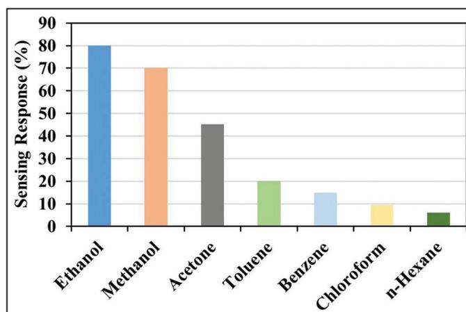
**Figure 8:** The sensing response (%) of PPy/SnO<sub>2</sub>/SWCNTs sensor towards different analyte vapours at room temperature. PPy: Polypyrrole, SnO<sub>2</sub>: Tin oxide, SWCNTs: Single-walled carbon nanotubes.
