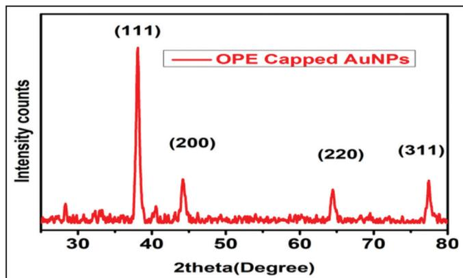
Figure 4: Powder X-ray powder diffraction pattern of orange (*Citrus sinensis*) peels extract capped gold nanoparticles.
