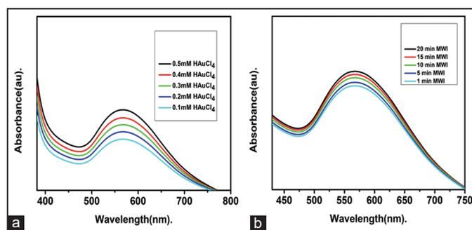
**Figure 1:** UV-visible spectra of synthesized gold nanoparticles (a) at different concentrations of chloroauric acid, (b) different microwave time irradiation.
