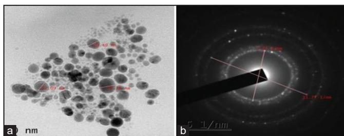
Figure 5: (a) Transmission electron microscopy image of orange (*Citrus sinensis*) peels extract capped gold nanoparticles and (b) corresponding SAED pattern.
