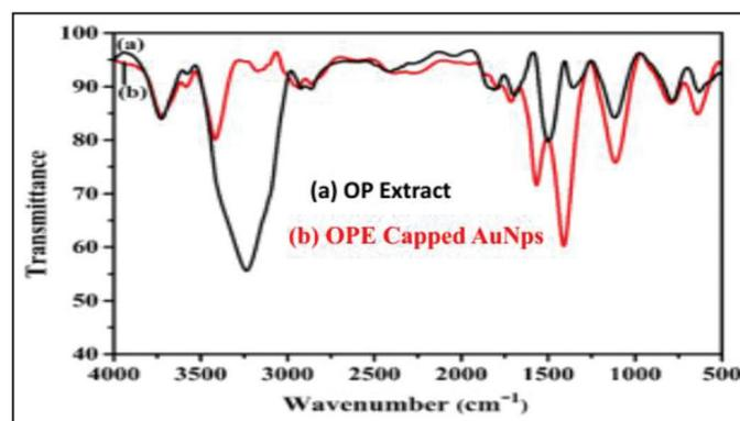
**Figure 2:** Fourier-transform infrared spectroscopy spectra of (a) orange (*Citrus sinensis*) peels extract and (b) orange (*C. sinensis*) peels extract capped gold nanoparticles.
