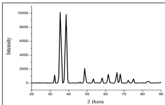
**Figure 1:** Powder X-ray diffraction spectrum for pure copper oxide nanoparticles.
