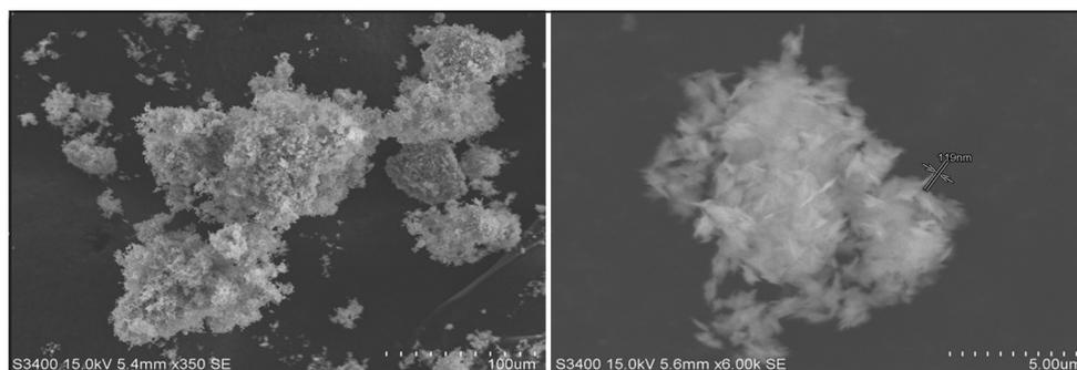
**Figure 2:** Scanning electron microscopy images for pure copper oxide nanoparticles.
