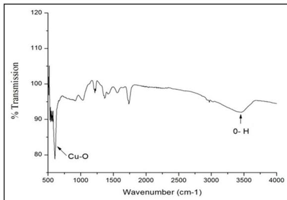
**Figure 3:** Fourier transform infrared spectra of the prepared copper oxide nanomaterial.
