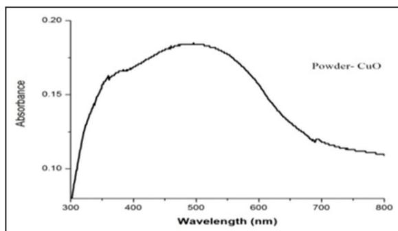
**Figure 4:** Ultraviolet-visible spectra of copper oxide nanoparticles.
