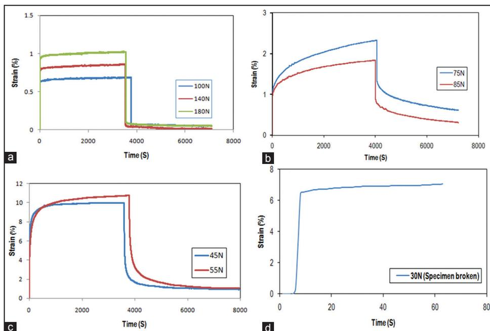
**Figure 2:** Creep and recovery of epoxy shape memory polymers at different temperatures: (a) 25, (b) 80, (c) 103, and (d) 120°C.
