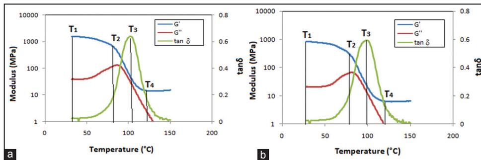
**Figure 1:** Advanced Rheometric Expansion System plots of: (a) Epoxy shape memory polymers (SMP) and (b) 5% carboxyl-terminated butadiene acrylonitrile-epoxy SMP.
