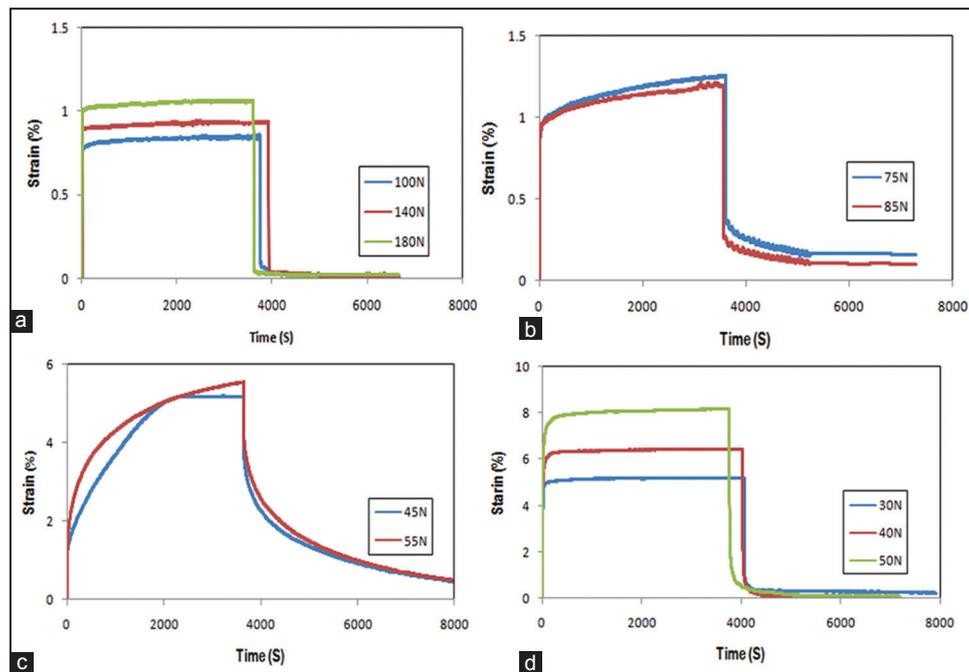
**Figure 3:** Creep and recovery of 5% carboxyl-terminated butadiene acrylonitrile-epoxy shape memory polymers at different temperatures: (a) 25°C, (b) 80°C, (c) 103°C, and (d) 120°C.
