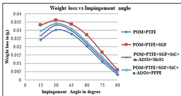
**Figure 1:** Depicts the weight loss of the polyoxymethylene/polytetrafluoroethylene composite versus impingement angle.
