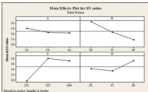
**Figure 2:** Main effects plot for signal-to-noise ratio of erosion test.
