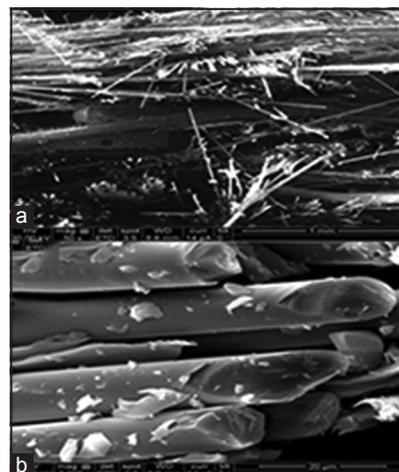
**Figure 6:** Scanning electron microscopy images of tensile fractured surface of GB-E samples: (a) At  $\times 50$  magnification; and (b) At  $\times 2000$  magnification.
