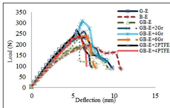
Figure 2: Typical load as a function of deflection of G-E, B-E and unfilled and filled GB-E composites.
