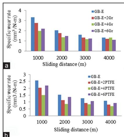
Figure 5: Variation in specific wear rate against sliding distance of unfilled GB-E and filled GB-E composites at 20 N.
