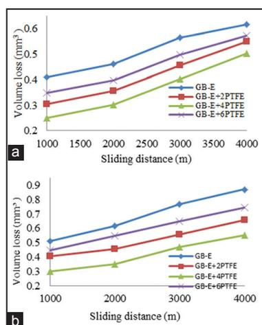
Figure 4: Wear volume loss of unfilled and polytetrafluoroethylene filled GB-E samples at (a) 10 N and (b) 20 N.
