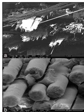
**Figure 7:** Scanning electron microscopy images of tensile fractured surface of GB-E+2Gr samples: (a) At  $\times 50$  magnification; and (b) At  $\times 2000$  magnification.
