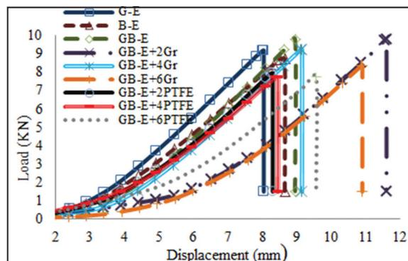
Figure 1: Typical load as a function of displacement of G-E, B-E and unfilled and filled GB-E composites.
