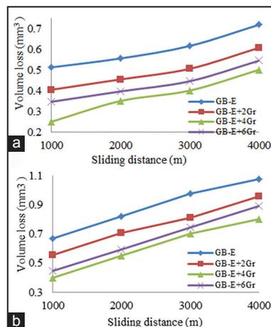
Figure 3: Wear volume loss of unfilled and graphite filled GB-E samples at (a) 10 N and (b) 20 N.
