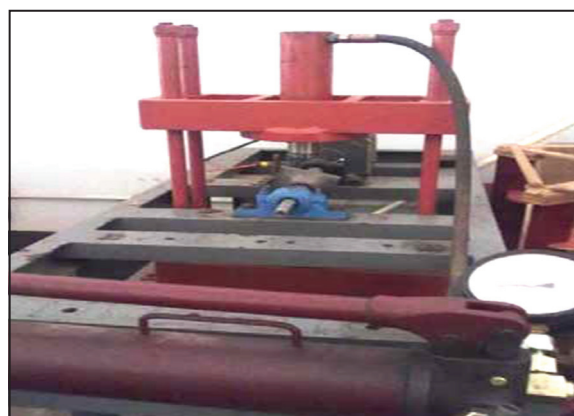
Figure 4: Experimental set up for vibration testing of bearing.
