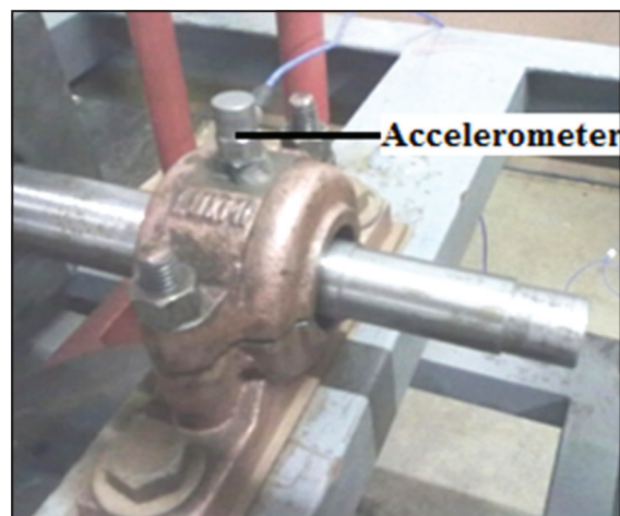
Figure 5: Accelerometer and mounted on bearing housing.
