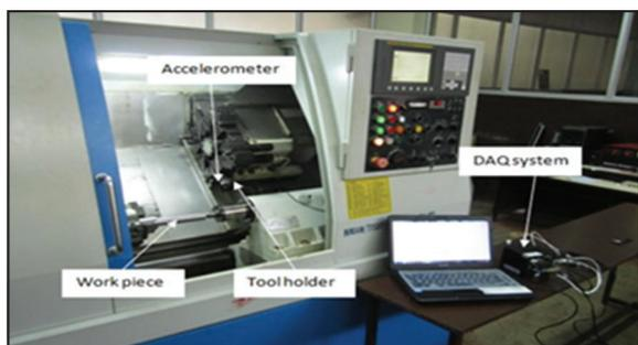
Figure 1: Experimental setup for measurement of cutting vibrations.
