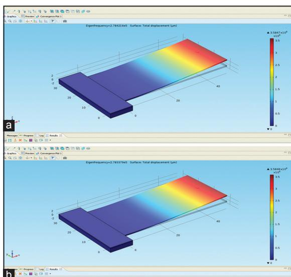
Figure 2: Simulated results at first mode of eigenfrequency for rectangular microcantilever for silicon material, (a) without mass, (b) with mass.
