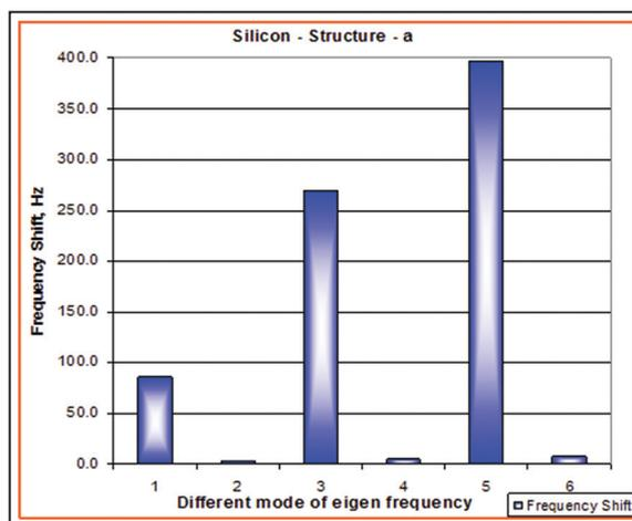
Figure 5: Frequency shift in each eigenfrequency mode (Structure A).
