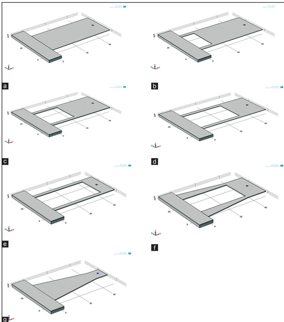
Figure 1: (a-g) Different structures of microcantilever.
