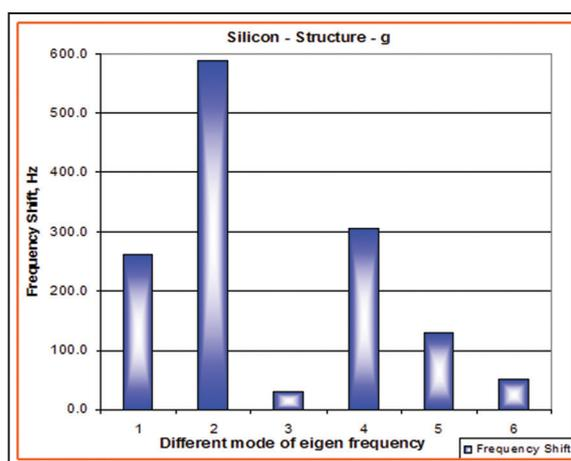
Figure 6: Frequency shift in each eigenfrequency mode (Structure G).
