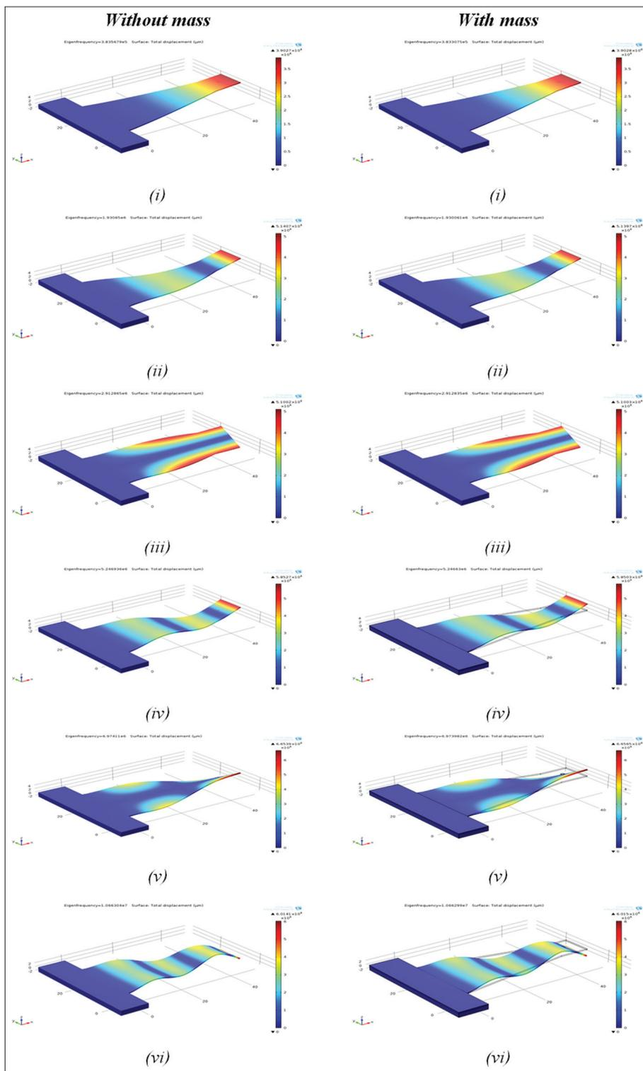
**Figure 4:** (i-vi) Simulated results at six modes of eigenfrequencies for trapezoid microcantilever without and with mass.
