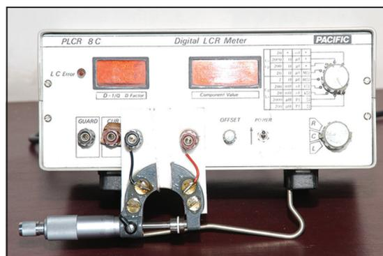
**Figure 4:** Experimental set-up for the determination of bone electrical and dielectric properties.
