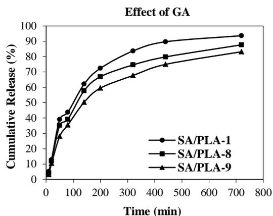
**Figure 6(c):** % of Cumulative release of Penicillamine through SA/PLA blend membranes containing different amounts of cross-linking agent.
