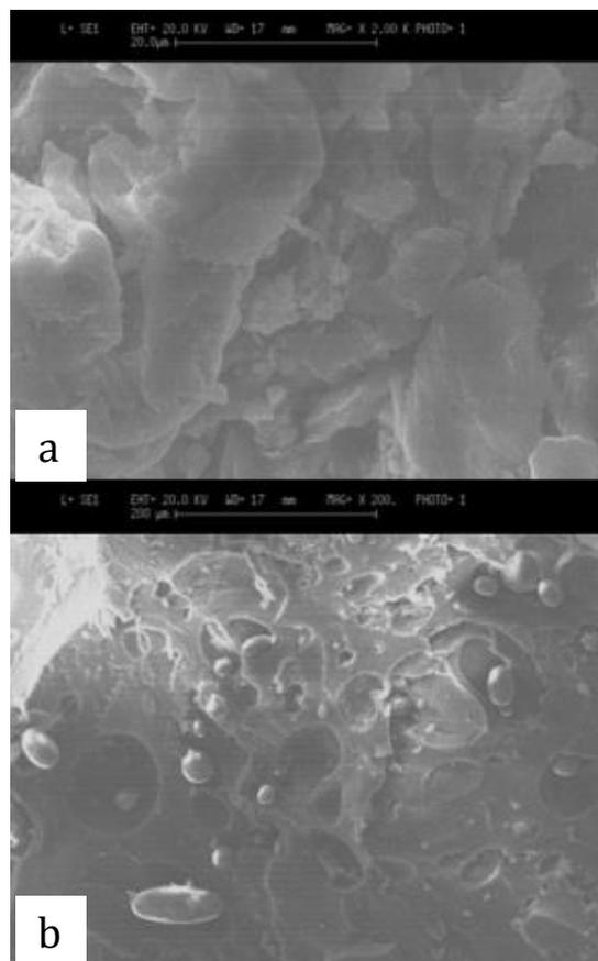
**Figure 4.** SEM micrograms of plain blend membrane (a) and Penicillamine Loaded blend membrane (b)
