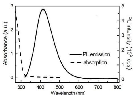
**Figure 3:** PL emission (solid line) and absorption (dashed line) spectra of the MPA-capped ZnS QDs with the ratio of MPA:Zn:S = 8:4:1.
