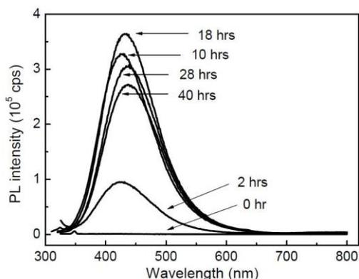
**Figure 5:** PL spectra of the MPA-capped ZnS QDs with MPA:Zn:S = 8:4:1 and synthesized at pH 8, after hydrothermal treatment at 100 °C for various period of time, i.e., 0 hr (no heat treatment), 2 hrs, 10 hrs, 18 hrs, 28 hrs, and 40 hrs.
