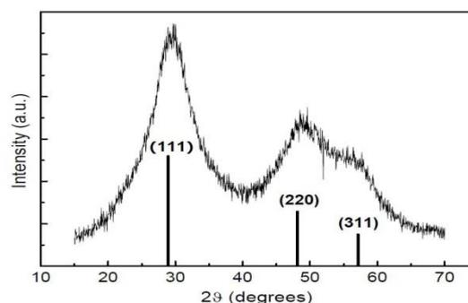
**Figure 2:** XRD pattern of the MPA-capped ZnS QDs with a ratio of MPA:Zn:S = 8:4:1. The vertical lines indicate the pattern and relative intensities of bulk ZnS with cubic zinc blende structure.
