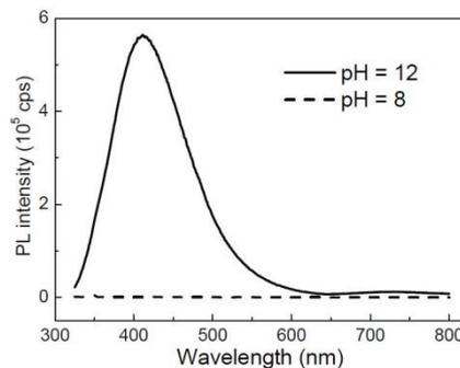
**Figure 4:** PL spectra of the MPA-capped ZnS QDs with the same ratio of MPA:Zn:S = 8:4:1, but synthesized at different pH, 12 (solid line) and 8 (dashed line).
