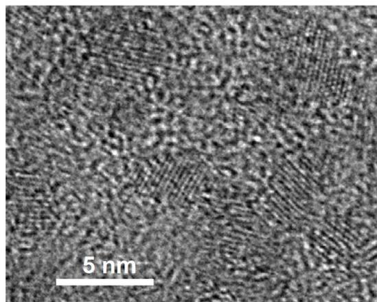
**Figure 1:** TEM micrograph of the MPA-capped ZnS QDs with a MPA:Zn:S ratio of 8:4:1.
