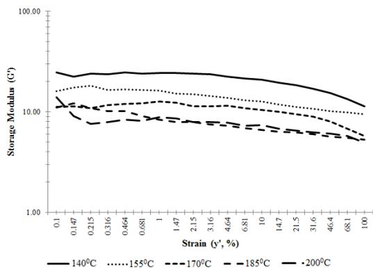
**Figure 7:** Plot of storage modulus ( $G'$ ) vs strain (%) obtained for the polyamide HMA at different temperatures.
