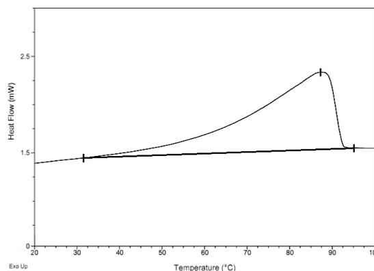
**Figure 4:** Cooling curve obtained for the polyamide HMA using differential scanning calorimetry.
