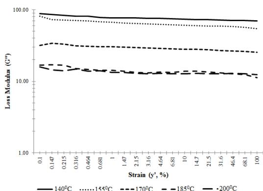
**Figure 8:** Plot of loss modulus ( $G''$ ) vs strain (%) obtained for the polyamide HMA at different temperatures.
