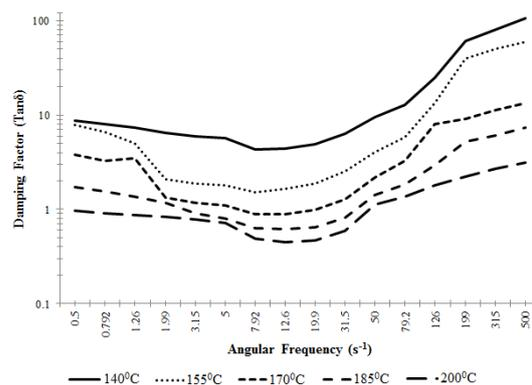
**Figure 10:** Plot of damping factor ( $Tan\delta$ ) vs angular frequency ( $s^{-1}$ ) obtained for the polyamide HMA at different temperatures.
