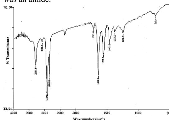
**Figure 2:** FTIR spectra obtained for the prepared polyamide HMA.
