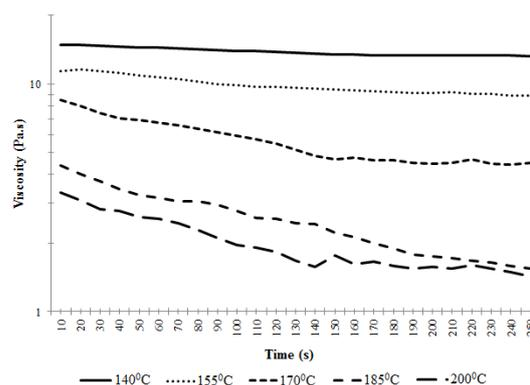
**Figure 6:** Plot of viscosity (Pa.s) vs time (s) obtained for the polyamide HMA at different temperatures.
