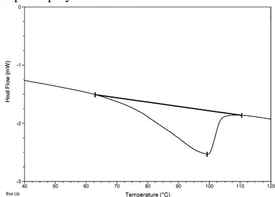
**Figure 3:** Heating curve obtained for the polyamide HMA using differential scanning calorimetry.
