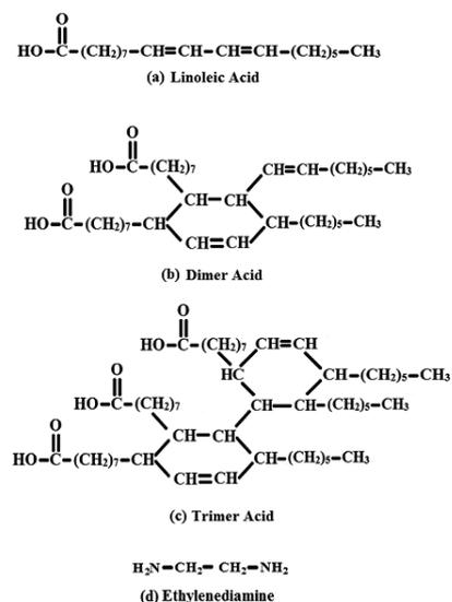
**Figure 1:** Molecular structure of the reactants used in the preparation of the polyamide HMA.
