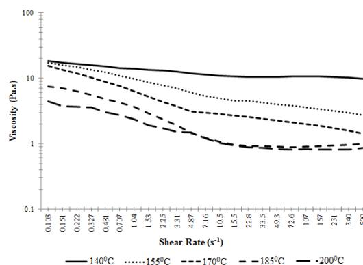
**Figure 5:** Plot of viscosity (Pa.s) vs shear rate ( $s^{-1}$ ) obtained for the polyamide HMA at different temperatures.
