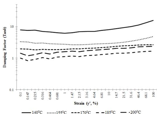
**Figure 9:** Plot of damping factor ( $Tan\delta$ ) vs strain (%) obtained for the polyamide HMA at different temperatures.
